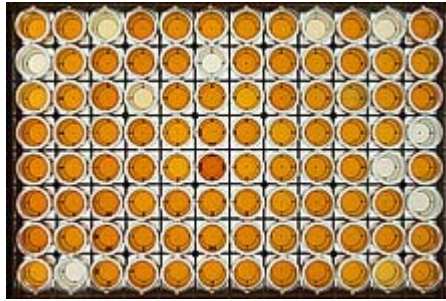
Fig. 17. A microtiter plate used to test plant samples for Xylella fastidiosa using enzyme-linked immunosorbent assay (ELISA). Each well represents one tree sample; a color change from clear to yellow indicates a test positive for the pathogen. (Courtesy A. B. Gould)
